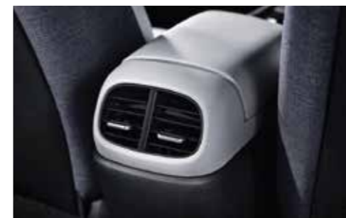
Rear Aircon Vent
